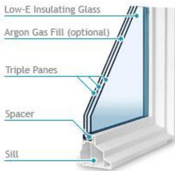
**TECHNOLOGY OVERVIEW** Triple pane windows use three panes of glass, usually with argon gas between panes to provide maximum energy efficiency and comfort. Window energy efficiency is measured using R
